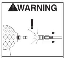
Always disconnect air from nailer whenever servicing! During maintenance, a nailer connected to air may fire accidentally, causing serious personal injury!
